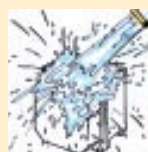
IP X5 Protection against jets of water from all directions
