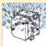
IP X3 Protection against rain (from an angle of up to 60^\circ to the vertical).
