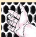
IP 1X Protection against access to dangerous parts with the back of the hand. Protection against solid foreign objects of diameter up to \geq 50 mm
