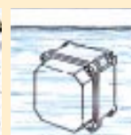
IP X7 Protection against damage by temporary immersion.
