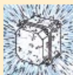
IP X4 Protection against splashed water (from all directions).
